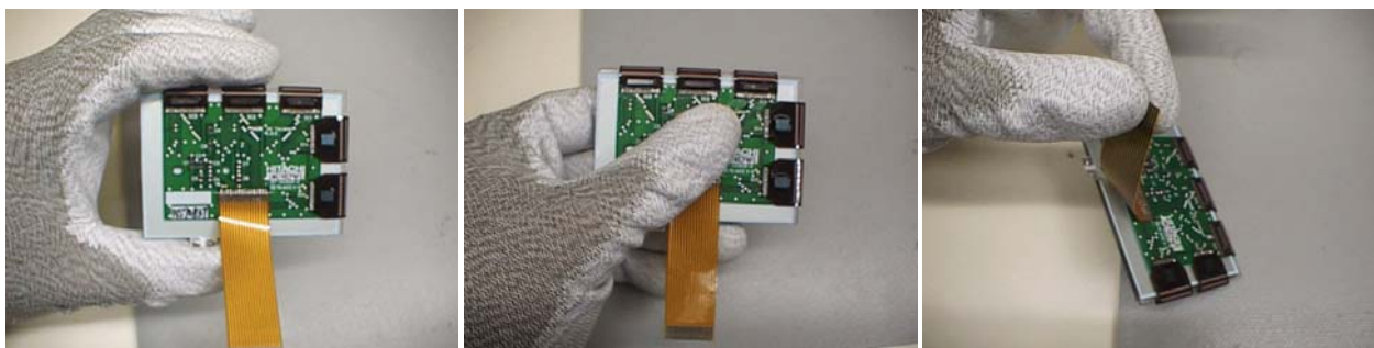
Figure 4: Incorrect Handling of the Liquid Crystal Module
